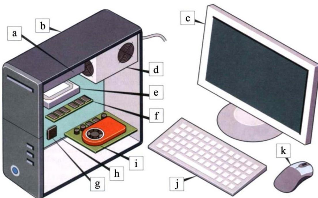
1) monitor, 2) case, 3) motherboard, 4) CPU, 5) main memory (RAM), 6) expansion cards (video, graphic), 7) power supply unit, 8) optical disk drive, 9) hard disk drive, 10) keyboard, 11) mouse
